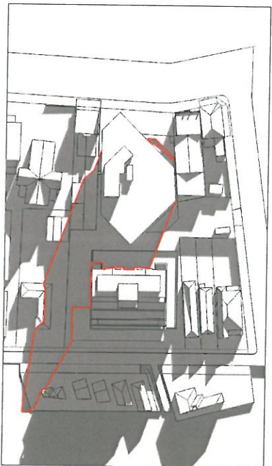
BUILDING ENVELOPE > EXISTING Winter Solstice, 21 June [9am]
