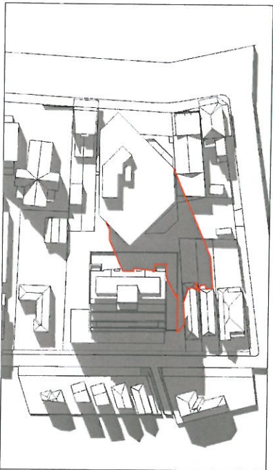
BUILDING ENVELOPE > EXISTING Winter Solstice, 21 June [12pm]
